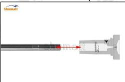
(5) When installing the injector valve assembly, the oil inlet position should be 180° between the oil inlet position of the injector body.
