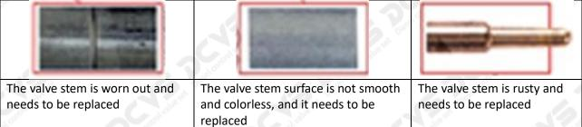
The excessive clearance between the valve stem wear, housing and the valve cap will causes injector lag.
